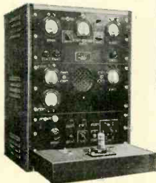
R.F. Universal Power Output Test Set built for Evans Signal Laboratories. Measurements from 20 to 4000 watts; from 2.5 mc to 60 mc.
