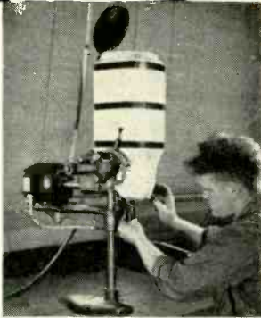
Robinson Metering Pump being used to forcibly eject metered amounts of cement into wire brush handle. Reservoir temperature 350° F.
